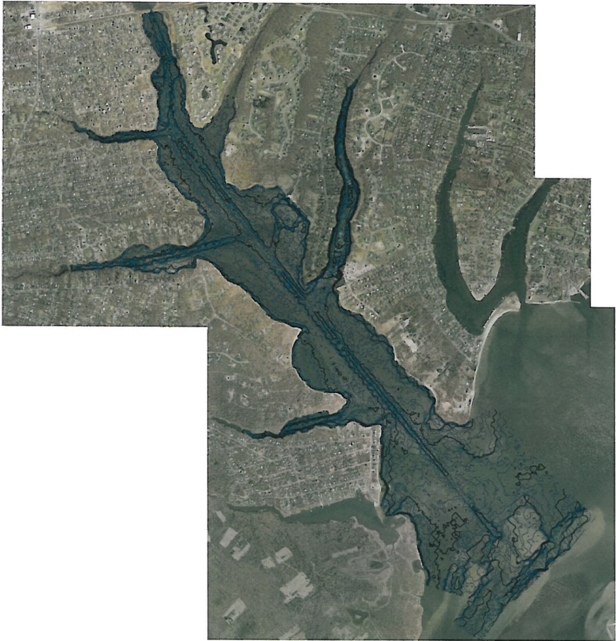
Figure 6. Bottom contours from Figure 5 plotted on 2004 air photographs downloaded the New York State GIS web site. The thicker contour lines are at 0.5 m depth intervals while the thinner contours are at 0.1 m depth intervals. The zero level of the contours is MLW_DB.
