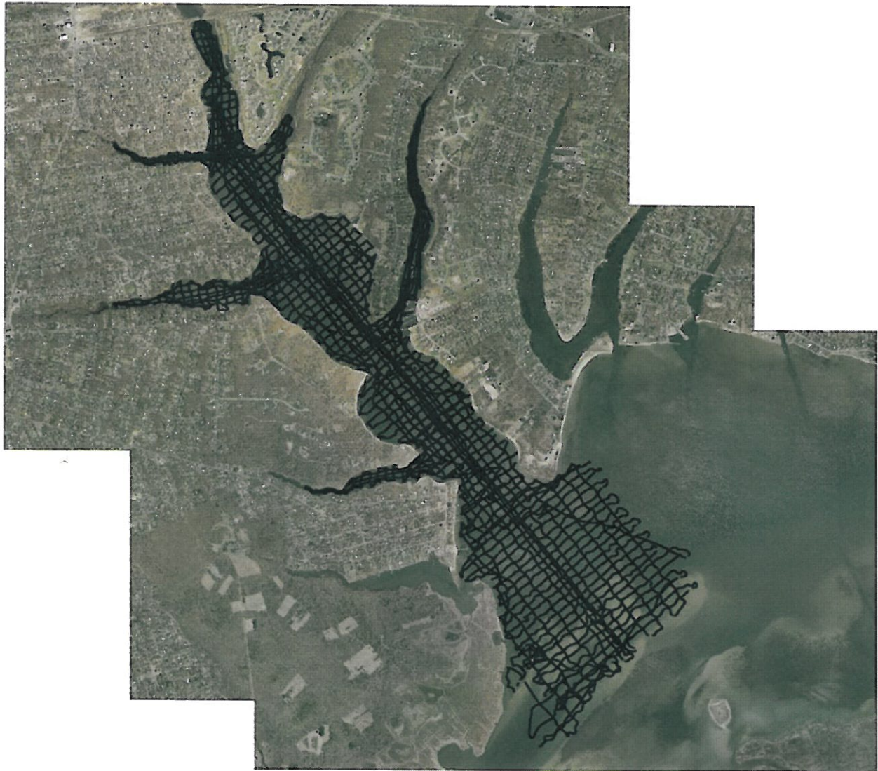
Figure 2. Survey tracks run on December 18, 30, 31 (2007) and January 8 (2008). All of the cross-channel lines and most of the along-channel lines were run. Depth data was collected while moving between lines as well as while running lines.
