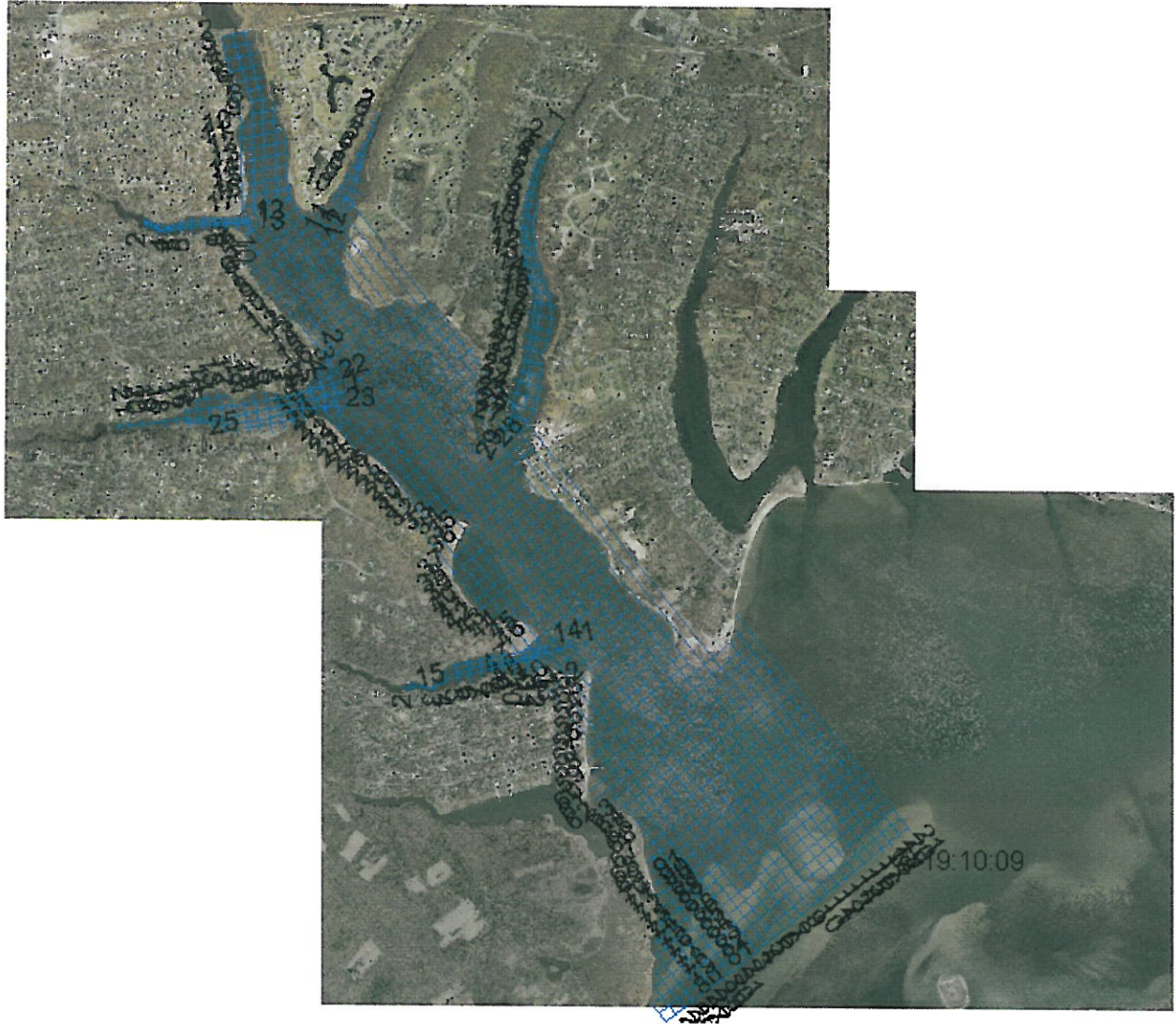
Figure 1. Planned survey tracks in the Forge River, although it may not be possible to run all of the tracks due to shallow water or obstructions. These tracks are spaced at 50 m intervals and run parallel to and perpendicular to the channels and tributaries. This grid of tracks will provide sufficient information to create a detailed picture of the sea-bed morphology in this region.
